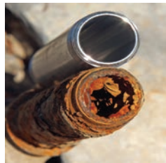
New galvanized pipe vs. buildup in galvanized pipe
